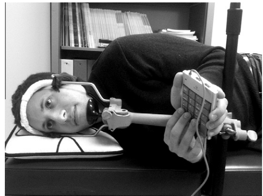
Fig. 2. A person fitted in the horizontally mounted head and chin rest with head strap holding a response pad as used in Experiment 1a.
